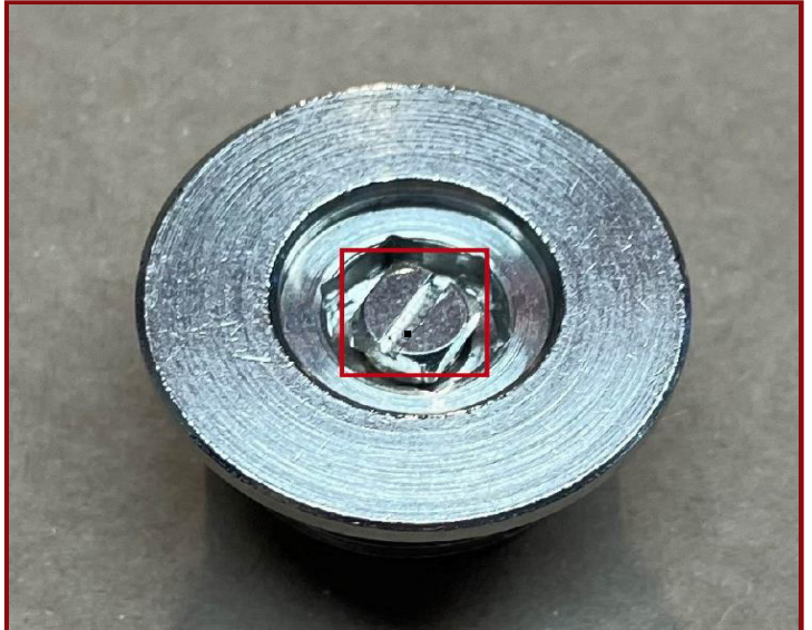
2 There is a small indentation in the air bleed screw
