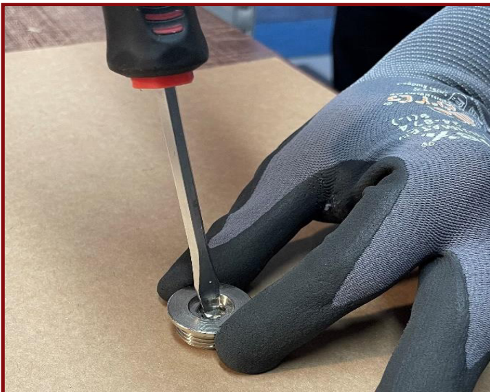
3 Use a flat head screwdriver or similar tool to turn the screw anti clockwise (about 1/4 turn)
